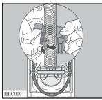
3. With a suitable spanner unscrew and remove the central rear bolt **A**. Slide out the relevant plastic spacer.
